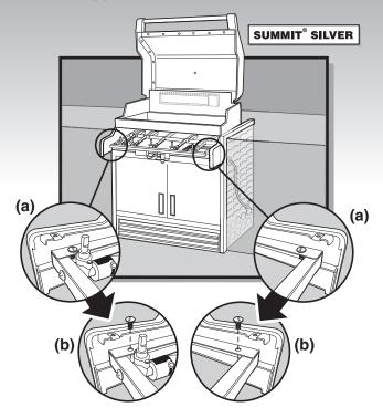
10. Pull manifold assembly out from the manifold frame.
